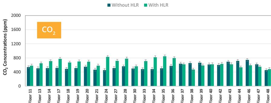
Figure 7: HLR technology maintains CO<sub>2</sub> below 850 ppm, well below the 1,100 ppm target. Lower set points can be enabled which will adjust adsorption and regeneration time.
